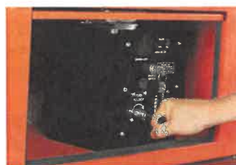
Remote control panel protected inside locked toolbox.
