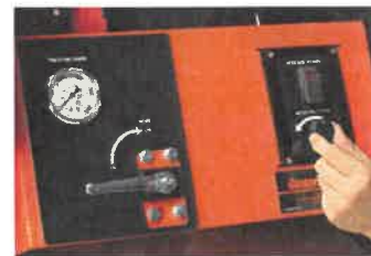
Easily accessible Variable Speed rewind control, along with pressure gauge and output valve mounted between hose reels.
